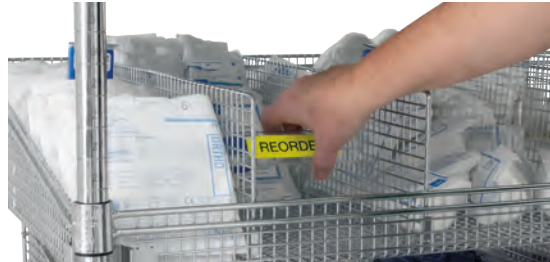
Lower Kanban Flipper to Signal to the Portal that Inventory Needs to be Replenished
